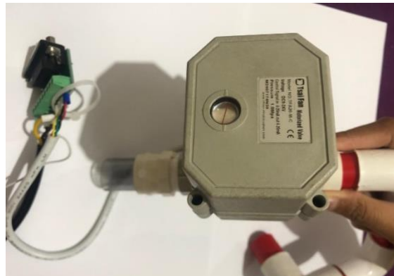
Gambar 14 Proses Pengujian Shut Down Valve (SDV)
